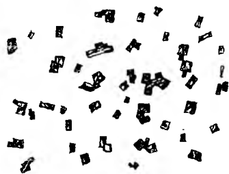
15-rasm. K_2SrCu(NO_2)_6 ning kristallari.
