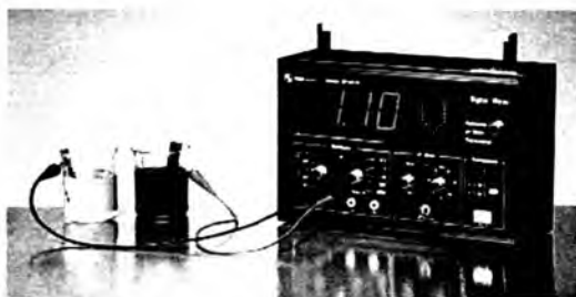
Tajriba: Galvanik element —elektr tokini o'lchovchi apparat Stakanlarda Rux sulfat (rangsiz) va mis sulfat (havorang) eritmasiga rux va mis elektrod tushirilgan 2-Raymond Chang, Kenneth A. Goldsby. CHEMISTRY, McGraw-Hill Education, USA, 2012 29 bet
